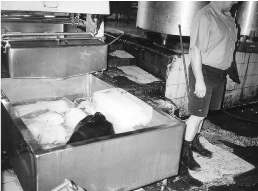
Ice will not chill the milk sufficiently during power shortages at this milk collection centre (Indonesia).
