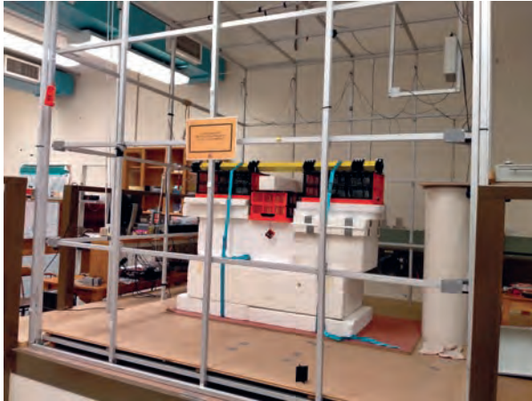
Fig. 5.13. Rubens cage in which the magnetometer was run along the yellow track above the rock cylinder sample carrying a magnetisation in the Black Hill Norite direction. The background field was set to be identical to the geomagnetic field at the Black Hill Norite location. The survey was performed by moving the sample perpendicular to the track after recording each flightline.
