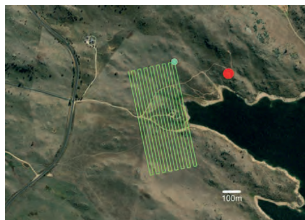
Fig. 10.18. Survey S2 flight lines. The red point is the ground station, the green point is the survey start location.
