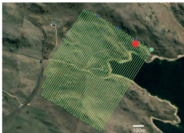
Fig. 10.17. Survey S1 flight lines. The red point is the ground station, the green point is the survey start location and the blue points mark survey breaks for battery replacement.
