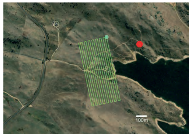
Fig. 10.18. Survey S2 flight lines. The red point is the ground station, the green point is the survey start location.
