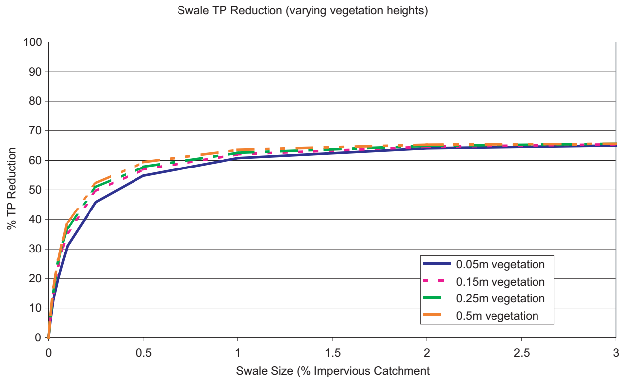
Figure 8.8 Performance of a swale in removing Total Phosphorus (TP) in Melbourne with varying vegetation height (channel slope = 3%).
